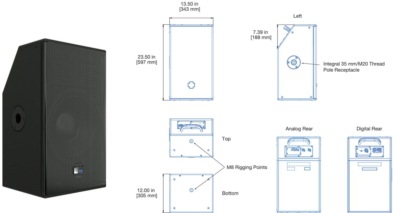
The USW-112P compact narrow subwoofer provides big bass sound for very tight spaces. Its compact rectangular enclosure and slanted connector panel enable flush-mounting of the cabinet against wall surfaces, reducing required installation depth to 12 inches, including connectors.
